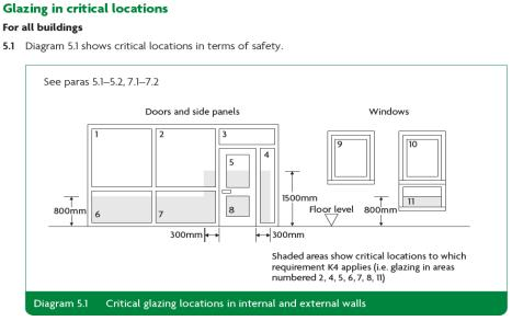
**Glazing in 'Critical Locations' should break safely,** i.e. laminated or toughened Class 2 safety glass complying with BS EN 12600 or Class C of BS6206. Or if it is installed in a door or in a door side panel and has a pane exceeding 900mm it should be Class 2 safety glass complying with BS EN 12600 or Class B of BS6206.
